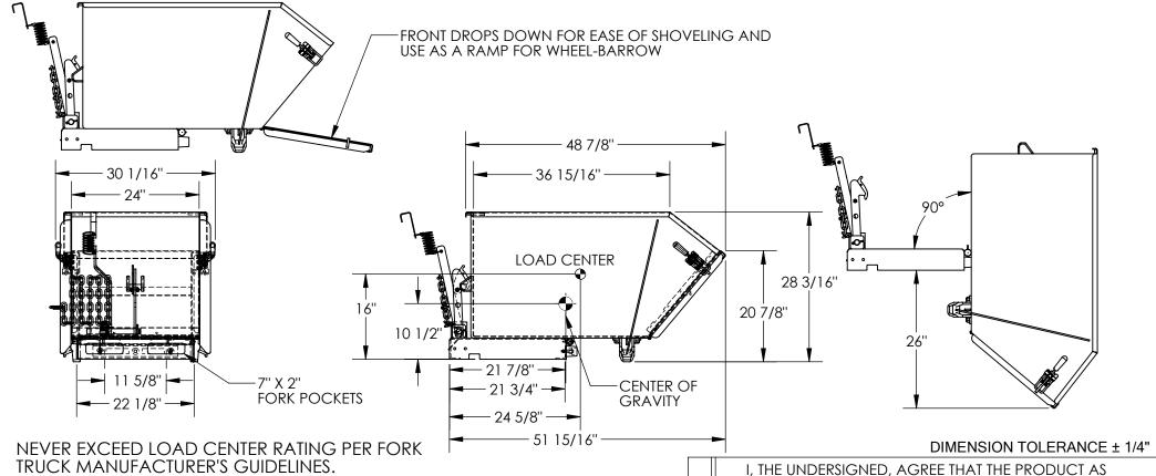
DO NOT USE THIS FORK TRUCK ATTACHMENT IF LOAD WILL EXCEED FORK TRUCK MANUFACTURER'S LOAD CENTER RATING. APPROX. WEIGHT/ LOST LOAD=281.01 LBS.
